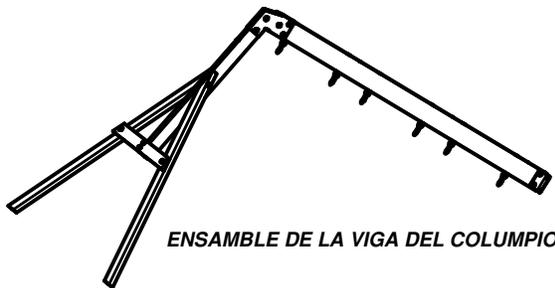
ENSAMBLE DE LA VIGA DEL COLUMPIO
