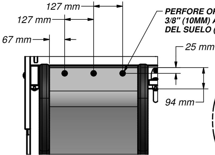
PERFORE ORIFICIOS DE 3/8" (10MM) A TRAVÉS DEL SUELO (3 PLCS)
